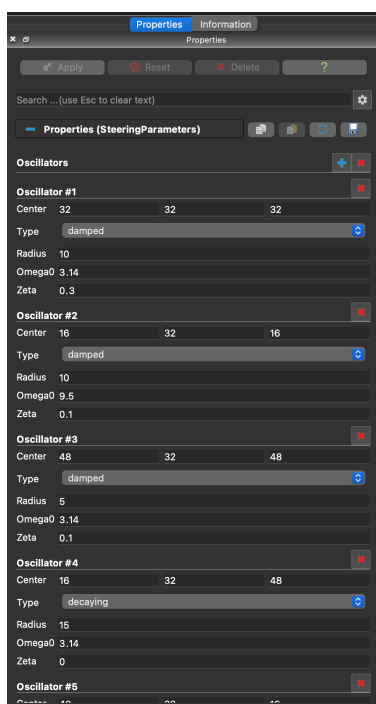
Fig. 4.17: The Properties panel provides parameters to add or delete oscillators in the domain, and change the parameters of the oscillators independently.
